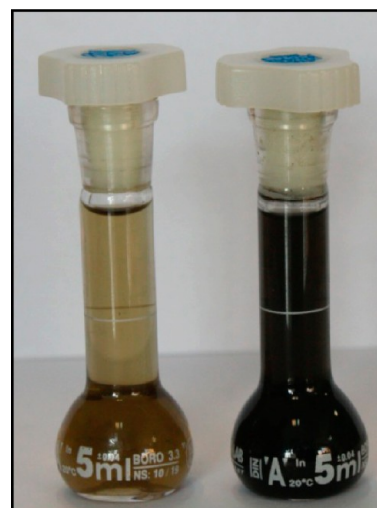
Figure 1. Digital photograph of Pt/Pd/Fe (1:1:2) T-NPs before (left-hand) and after (right-hand) reduction with hydrazine hydrate.
